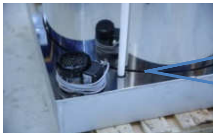
This special gasket will avoid any introduction in the water reserv.
